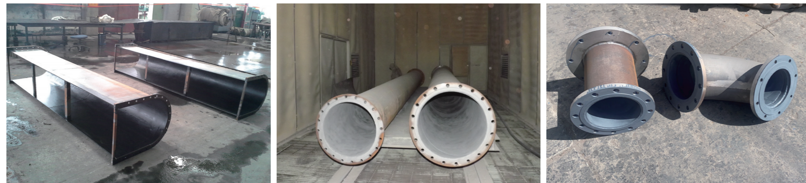
溜槽准备衬胶 Ready for lining
